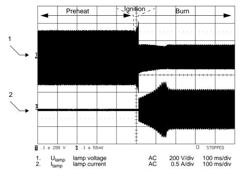
Fig.4 Lamp Voltage and -Current Delayed with 1.3 s
