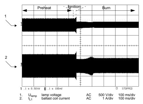
Fig.6 Ballast Coil Current Delayed with 1.3 s
